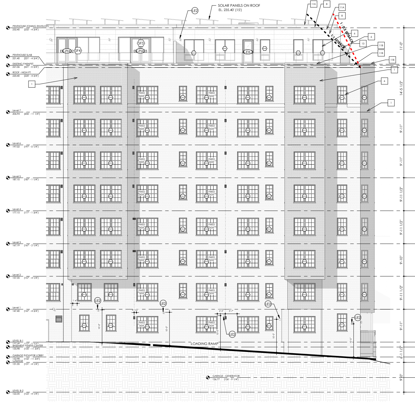
B5 PROPOSED - WEST ELEVATION - LOADING RAMP 1/8" = 1'-0"
